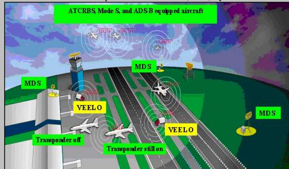
Multistatic Dependent Surveillance (MDS) System
