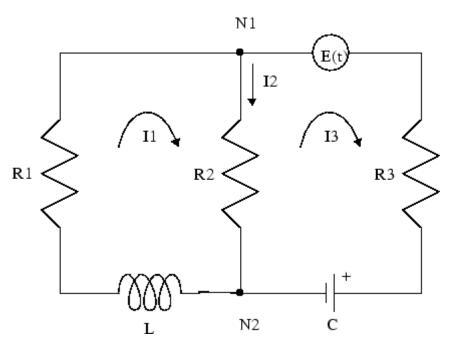
Let Rj and Ij, j = 1, 2, 3 be resistances (measured in ohms) and currents (amps), respectively; L be inductance (henrys), and C be capacitance (farads); E(t) be the electromotive force, and Q(t) be the charge.
