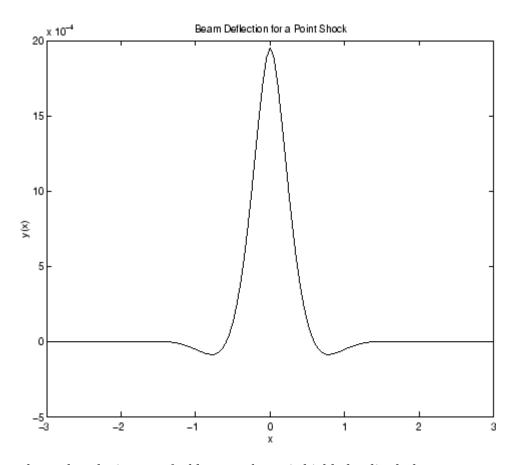
shows that the impact of a blow on a beam is highly localized; the greatest deflection occurs at the point of impact and falls off sharply from there. This is the behavior we expect from experience.
