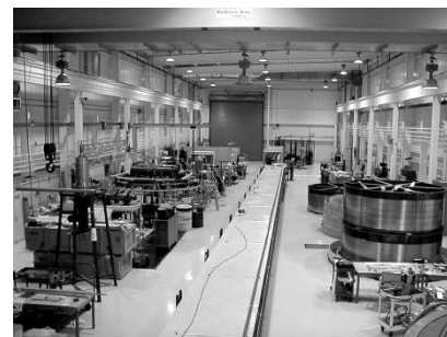
Fig. 4. SMES CICC fabrication line and coil assembly.
