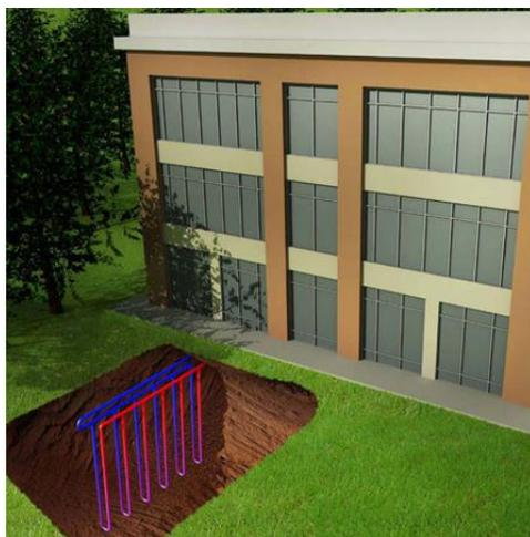
Figure C-1: Vertical bore fields can be up to 400 feet deep.\
