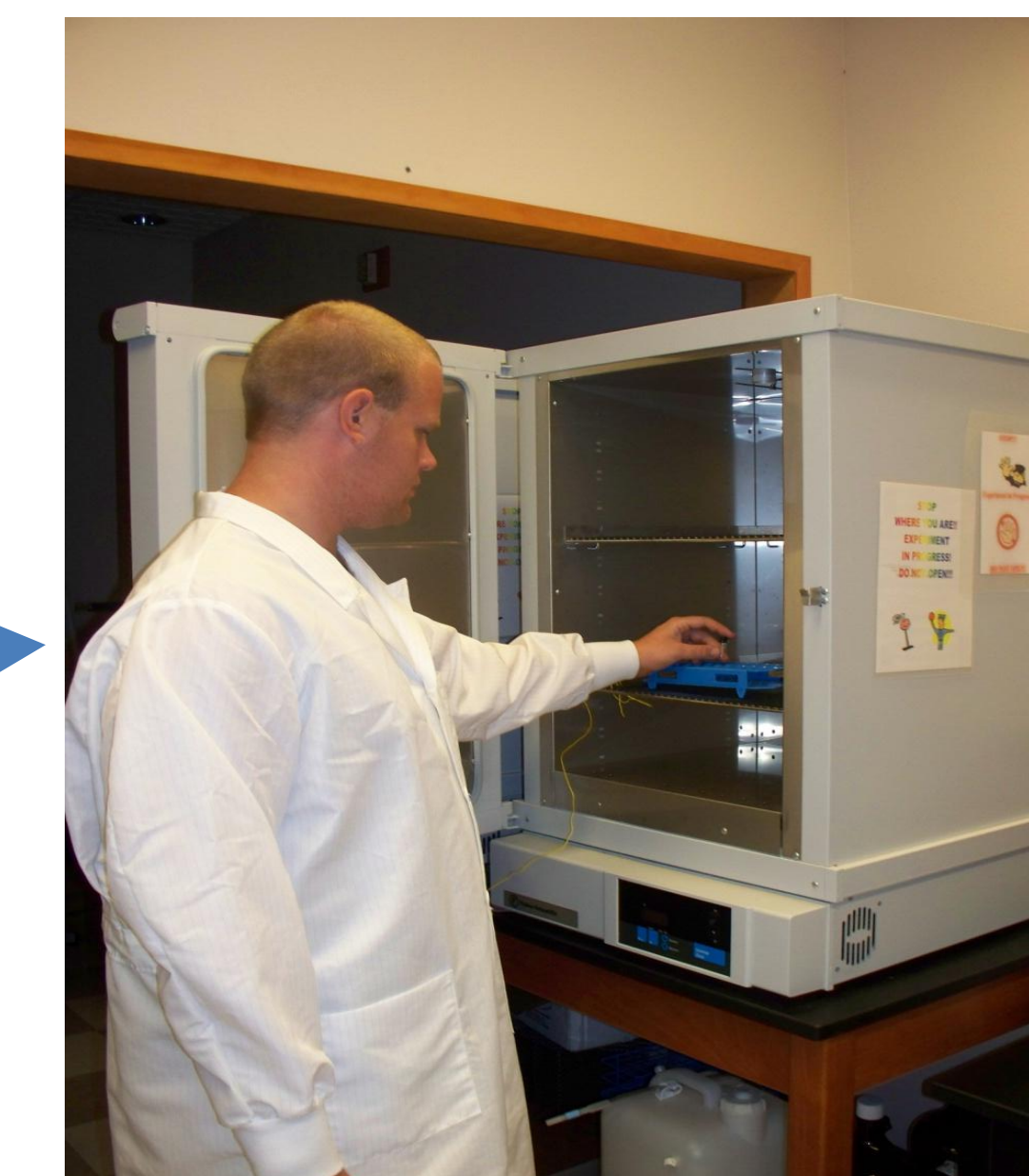
mix the sample and put into an isotemp oven for 1 hour at 85 degrees Celsius
