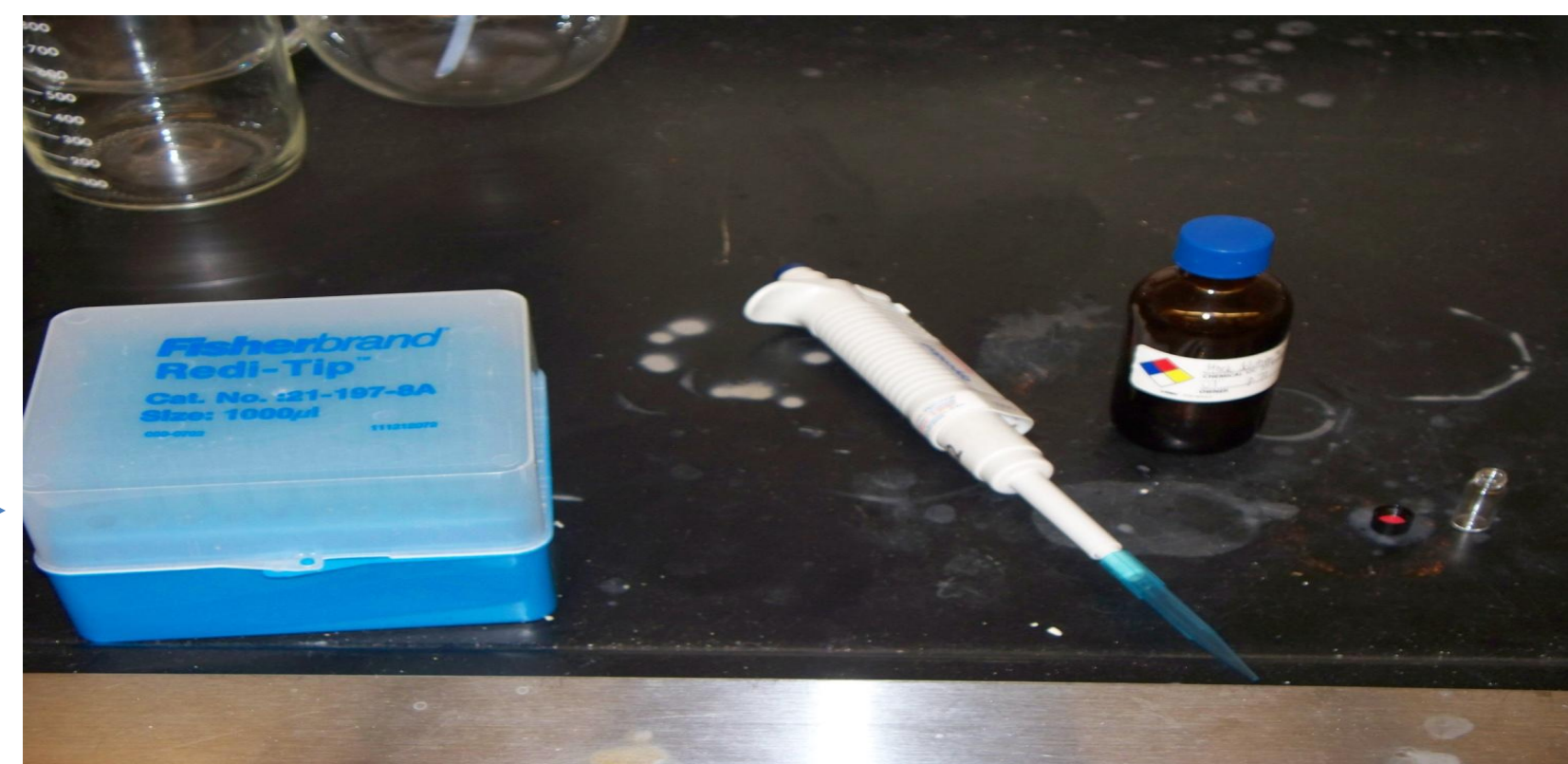
add .5 mL of a 1 microgram 2,4,6 trimethyl pyridine (TMP) / 1 mL methylene chloride solution (called stock solution #2) and seal
