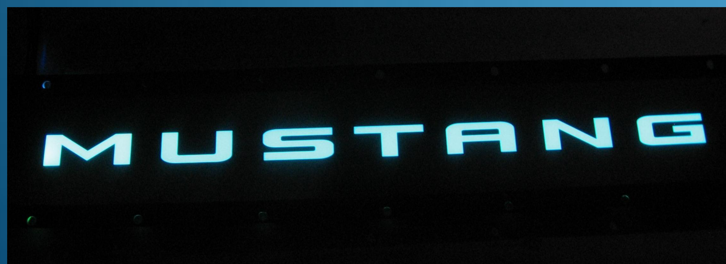
A finished part, partially assembled and lit by blue & green LEDs.
