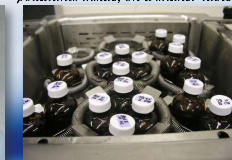
Batch reactors, with charcoal and pollutants inside, on a shaker table.
