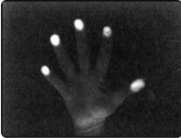
Figure 13: Example of finger touches on an FTIR screen 13
